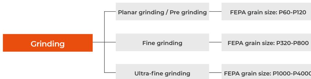
Typically, silicon carbide (SiC), aluminum dioxide (Al<sub>2</sub>O<sub>3</sub>), silicon dioxide (SiO<sub>2</sub>), zirconium dioxide (ZrO<sub>2</sub>), diamond or cubic boron nitride (CBN) are used as abrasives. Particular attention must be paid here to low-deformation material removal and at the same time to keeping the number of preparation steps as low as possible. A wide range of QPREP grinding media is available for this purpose.
