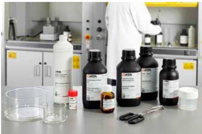
QATM offers a wide range of etchants for contrasting as well as for qualitative and quantitative analysis of microstructures. Different QPREP etchants are available for macro and micro etching as well as electrolytic etching.
