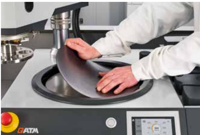
Applying the magnetic foil
