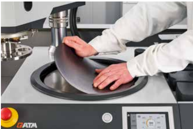
Applying the magnetic foil
