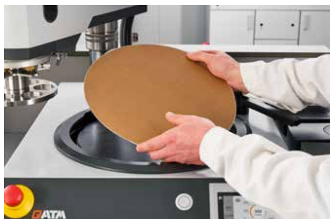
Applying GALAXY X-Tap on magnetic foil
