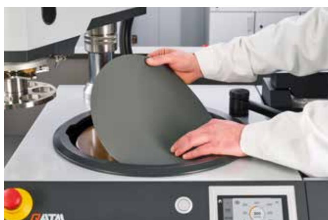
Placing e.g. self-adhesive grinding paper on GALAXY X-Tap
