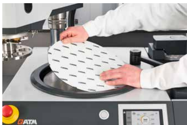
Applying the adhesive carrier disc
