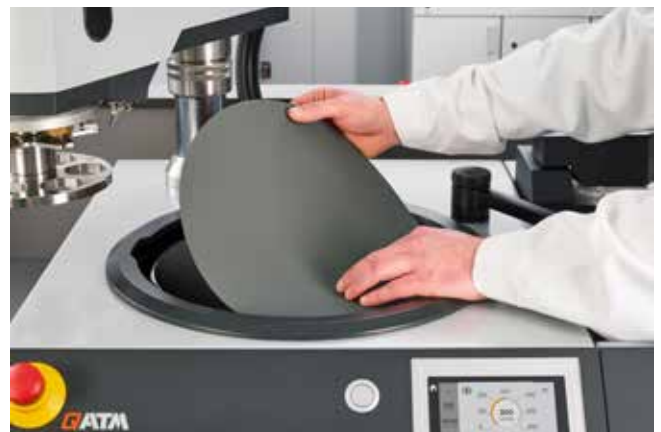
Placing e.g. grinding paper without adhesive/foil backing on Quick-Tap
