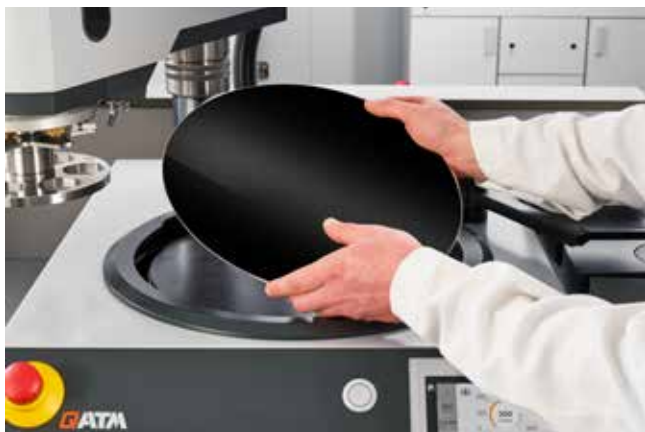
Applying Quick-Tap on magnetic foil
