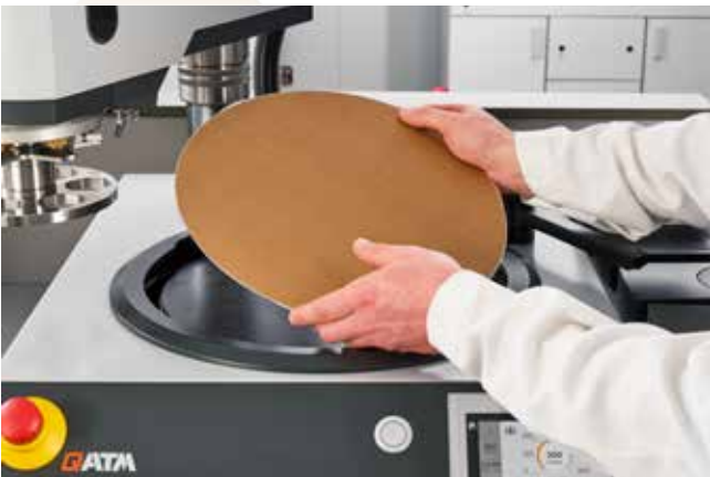
Applying GALAXY X-Tap on magnetic foil
