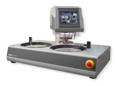
The **SAPHIR 560 WITH RUBIN 520** is a twin wheel grinder and polisher of recent generation with an innovative grinding and polishing head for working wheels Ø 250 - 300 mm. The grinding and polishing head 520 is equipped with an automatic protective hood and sets a new standard for operational safety.
