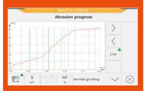
The grinding process is continuously monitored and graphically displayed using the SmartGrind software function.
