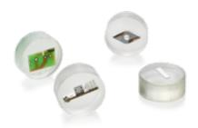
The Qmount is a modern device for the light-curing-based mounting of materialographic samples.
