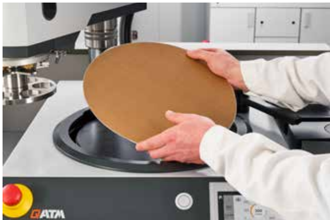
Applying GALAXY X-Tap on magnetic foil
