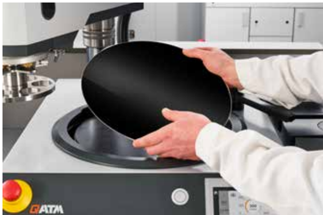
Applying GALAXY Quick-Tap on magnetic foil
