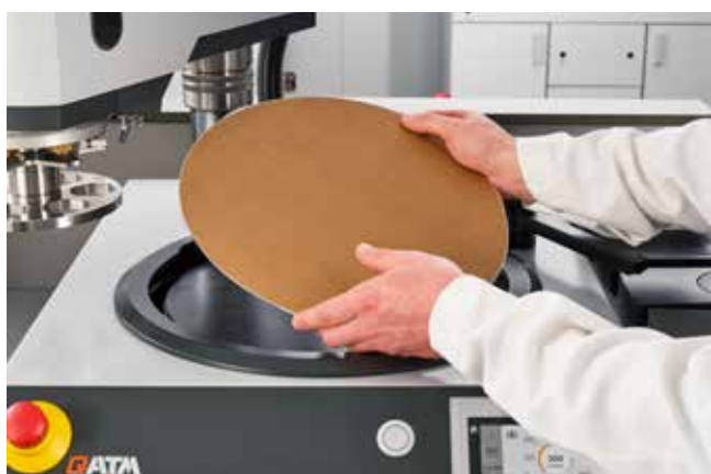
Applying GALAXY X-Tap on magnetic foil
